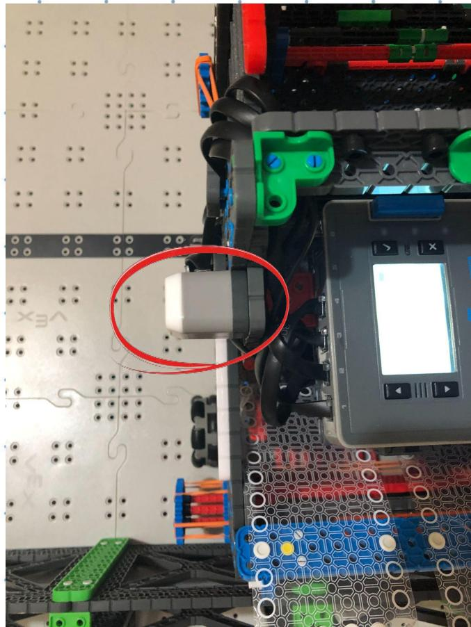
The LED sensor is on the side of our robot. We use it when starting a program. When the red light goes on, it means the gyro sensor is still calibrating. When the light turns green, it means the program is ready to start. It's easier to start a program with the LED.
