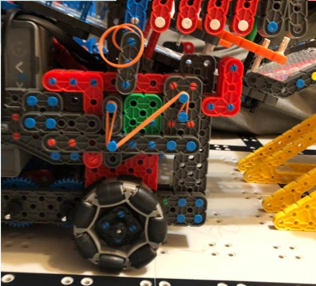
When the small red "L" piece comes into contact with the wall of the divider, the mechanism will shoot out onto the green section of the board. This mechanism will only be used at the end of each run. During the designing process of this mechanism, we realized that it wouldn't be very good if something were to accidentally hit the "L" piece, and release the long arm. So, we added extra locks (kind of like baby locks) that make sure they the arm goes out at the wrong time.
