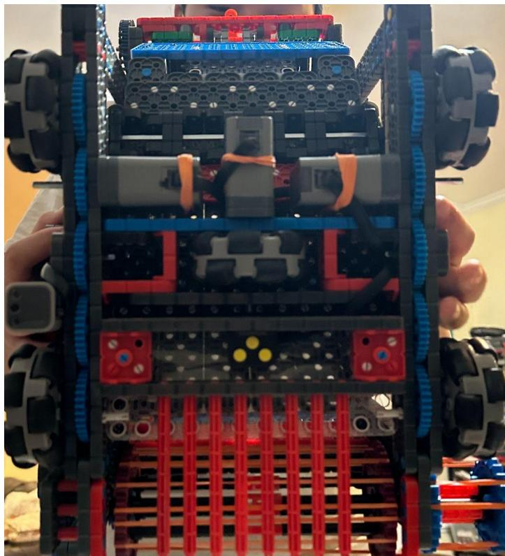
shift wheel is placed in the middle of the drivetrain horizontally to help the robot move from side to side for convenience.
