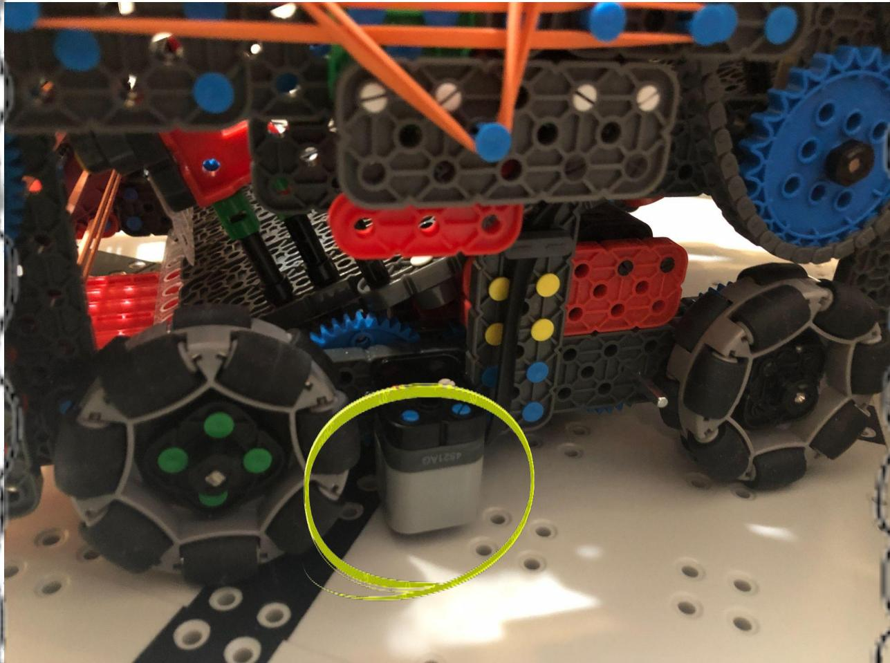
The color sensor sees black and white. We use it to make sure the robot drives straight while driving. We programmed it to make the robot drive on the black line, and since the black line is straight, the robot will drive straight. This allows more accuracy.
