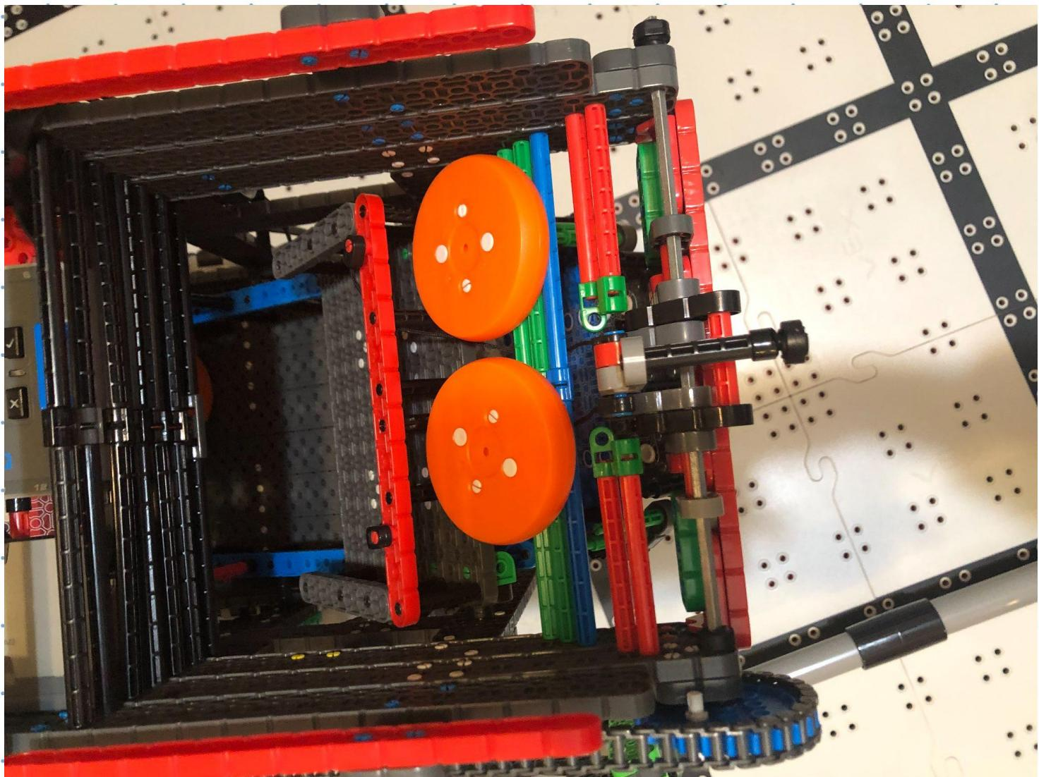
We encountered the problem of having the pucks fall into the wrong place. Instead of going onto the ramp, it gets stuck above the standoffs, causing it to get stuck. This problem only occurred while driving. After a few times we noticed that this occurred because we left the bottom layer ramp up in shooting position, letting the ramp have space to go down.
