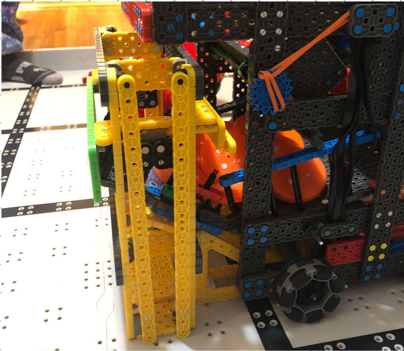
The ramp goes under the yellow dropper, hooks up, and the robot drives back. Then, the ramp goes down, holding all 9 pucks.
