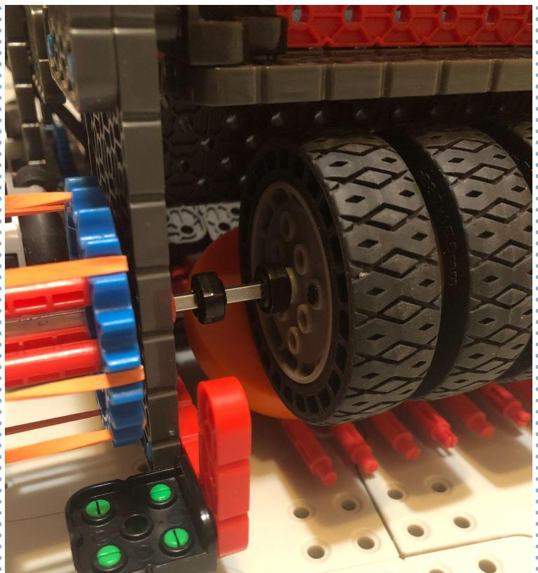
We decided to remove the section where the pucks fall into. Instead of having the pucks stack up into uniform columns, we changed the pucks to go straight into shooting. This way, we wouldn't have too much time spent on trying to load the pucks, and also we wouldn't have the problem of the pucks not loading into the columns in the correct orientation (the pucks can fall into the robot randomly, making it easier to avoid mistakes).
