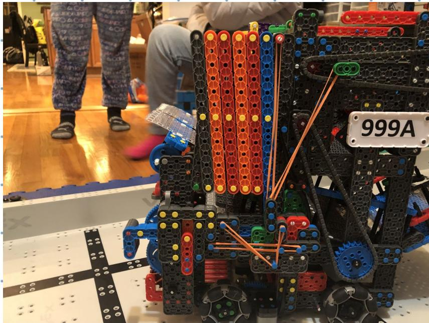
We had one motor that we could use, either for the shift wheel and touchdown motor. We had to make a tradeoff and decided to use it for the shift wheel.
