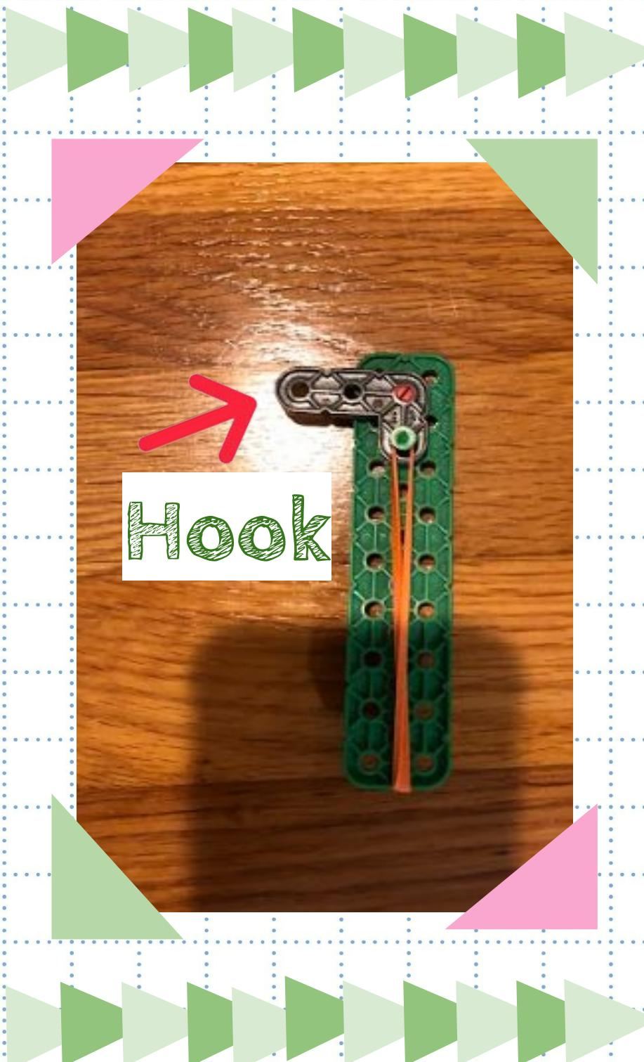
This hook design is made to drop the pucks from the yellow dropper. We plan to put it near the bucket. The robot drives behind the yellow dropper, then goes forward to hook onto it. The hook will have enough force to pull back the dropper so that pucks can fall into the robot. But the hook's rubber band tension is designed so that it can easily slide out of the dropper's edge.
