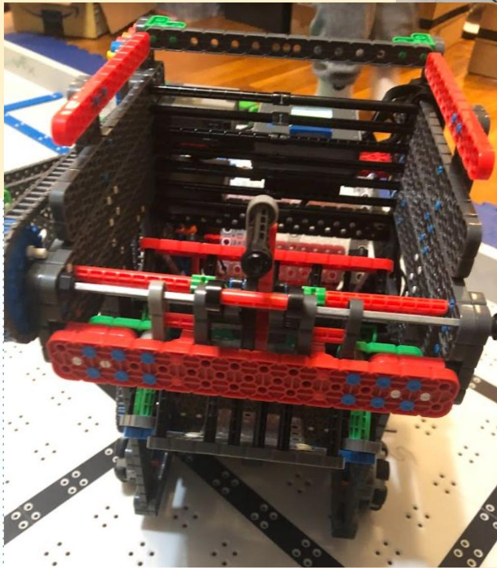
So, we made this design to save space, and make it more reliable. Also, it was easier to access the pucks on the blue dispensers due to the angle it and direction it moves.
