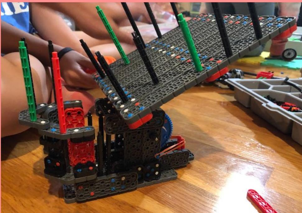
After trying the new design, and learning that it was successful, we attached the ramp we designed last week onto it. The ramp is attached so that pucks can easily slide into the shooter.
