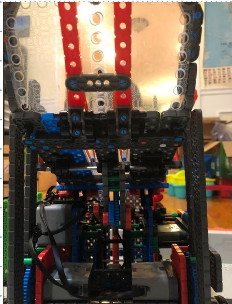
Before, our ramp design was not ideal, because it was flimsy. This design is sturdier than the first ramp we made. The beams are supported with more pieces, so that it can't be moved easily. Previously, the ramp would wobble from side to side, but now the ramp is stationary and more consistent. This ramp will be better than the old one because pieces won't easily fall off and the pucks will not roll off the ramp.
