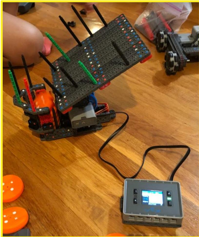
This design was made up of many 2x bars. The stand offs were added to lead the pucks into the shooter. We were planning to have the pucks drop onto the ramp, then roll into the shooter. There were a few problems with this design:
