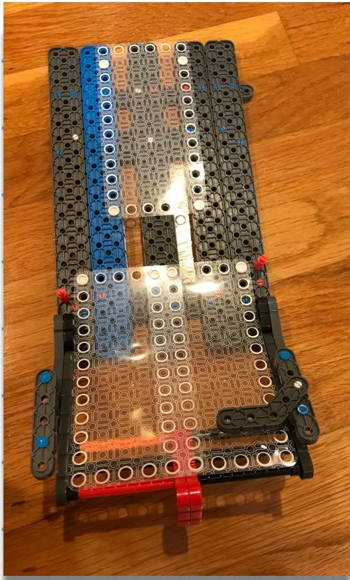
This design works just like the previous double hook. The only difference is that it is attached to the disk ramp and it is hooked on both sides. This allows the hook to hook down onto the blue disk dispenser and also hook the other way onto the yellow disk dispenser.
